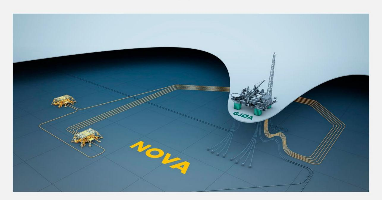
The Plan for Development and Operation for Nova is approved. The development solution involves two subsea templates tied back to the nearby Gjøa platform in the northern North Sea.
